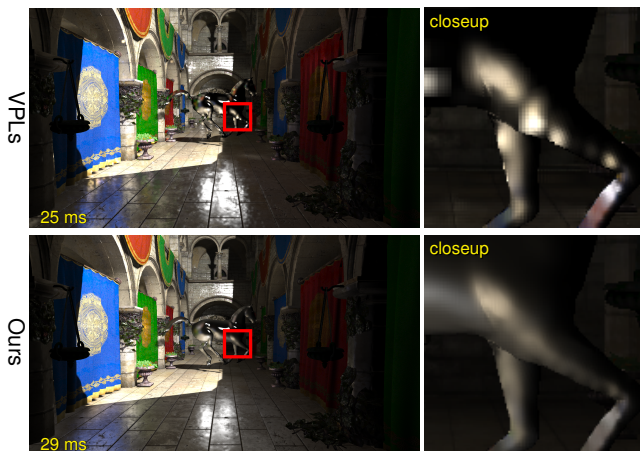
Figure 5: Textured scene with normal maps (The same scene as Fig. 1, Phong exponent: 1023). Using filtered VSGLs, spiky artifacts and temporal flickering are reduced significantly.
