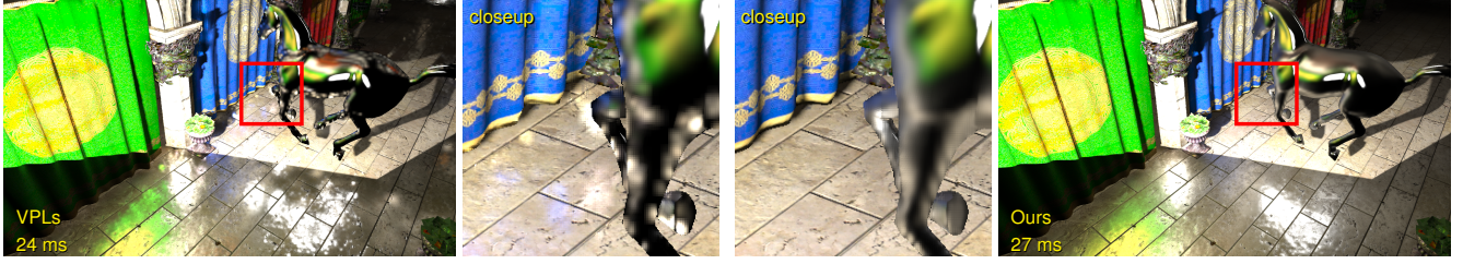
Figure 1: VPLs (left) and our method (right) for a dynamic scene (264465 triangles). VPLs produce spiky artifacts and temporal flickering, while our method suppresses these artifacts for all-frequency materials with 3 ms overhead (GPU: AMD Radeon™ HD 6990).
